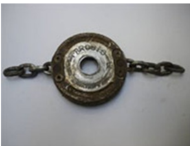
Chain flail attachment with two chains
